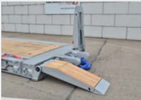
Single ramp for front loading
