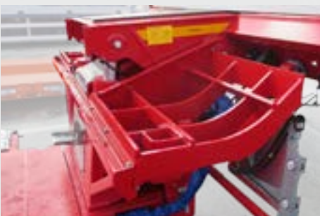
Wheel recess on the gooseneck
