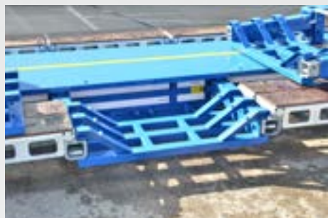
Lightweight pivotable wheel-wells
