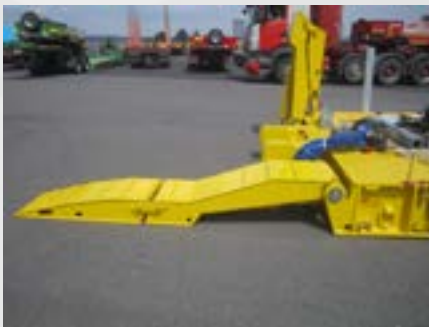
Double ramp for front loading
