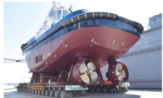
**AREKET** is putting its mark on many important projects, and one of them, it performed transportation of 6 vessel trailers for Uzmanlar Gemi. 33M x 9m x 17m sized trailers weighing 660 tonnes were transported from the Başiskele Free Zone to the pool at Uzmar Shipyard. During the transportation, HAREKET used 2x16 axle SPMT flatbed trailers and 2xPPUs and it also used a 400 tonnes crawler crane. While the first transports started in March 2018, the last transport was carried out in June.
